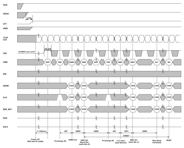
$<sup>^{\</sup>star}$  200 cycle(tXSRD) of CK are required (for DLL locking) before Read Command
